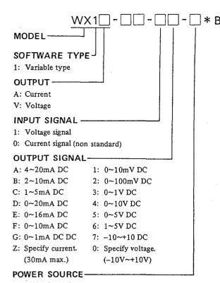
Ordering Information Measuring Range of Input Voltage input signal: 2V min. Span for 0~10V DC Current input signal (input resist:  $250\Omega$ ):  $(250\Omega)$  x (Input current) shall be within the measuring span of voltage input signals Recommended Range 4~20mA DC 2~10mA DC Current signal 0~20mA DC 0~16mA DC 0~10mA DC 0~10V DC Voltage signal 0~ 5V DC 1~ 5V DC
